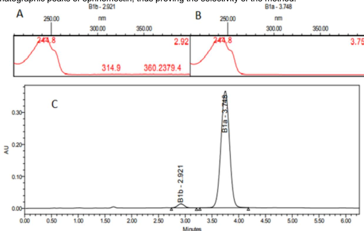
**Figure 2.** High-performance liquid chromatographic analysis, at  $\lambda = 245$  nm, showing the specificity of the method for eprinomectin (EPR) at concentration of  $300 \mu\text{g/mL}$  (B1b + B1a): (A) B1b peak scan spectrum; (B) B1a peak scan spectrum; (C) The chromatogram showing the EPR peaks B1b (2.921 min) and B1a (3.748 min).
