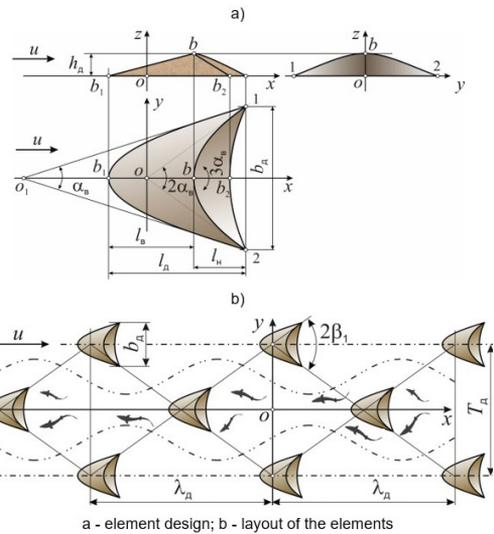
**Figure 1.** The dune-type flow-forming element design scheme.
