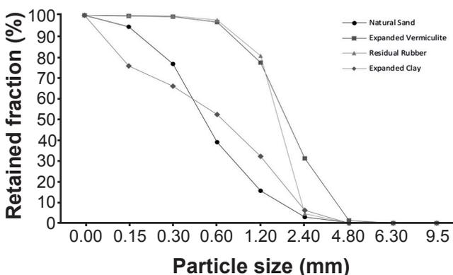
Figure 1: Granulometric curves of the aggregates used.
