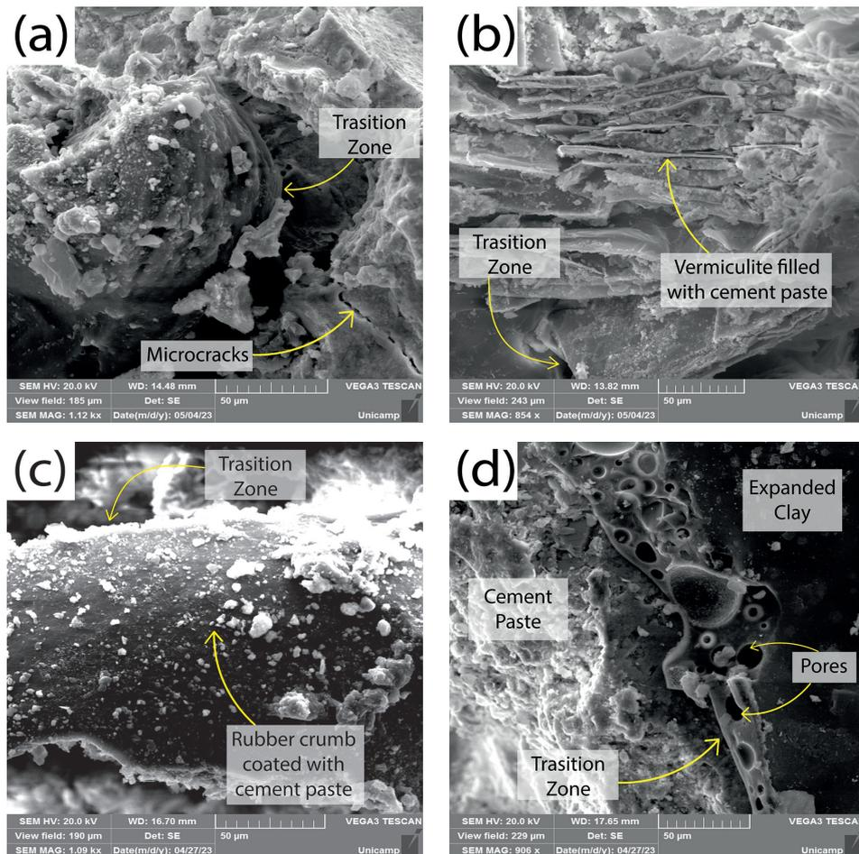
Figure 3: SEM micrographs of mortar samples: a) M25R-30EV-0EC; b) M35R-30EV-0EC; c) M25R-0EV-30EC; and d) M35R-0EV-30EC.
