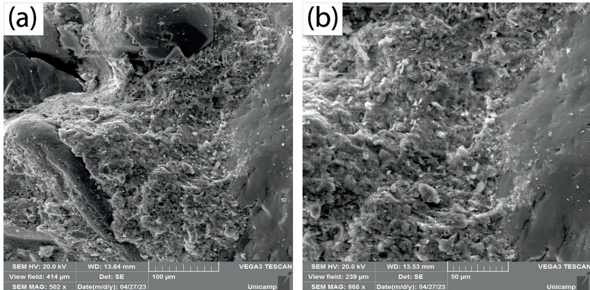
Figure 4: SEM micrographs of reference mortar sample M-0R-0EV-0EC at different magnifications.
