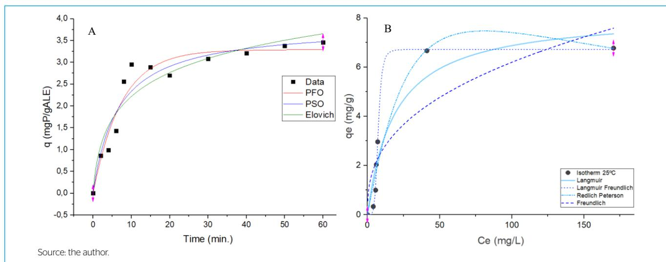
**Figure 4 - (A) Kinetic adsorption models; (B) fit of models applied to isotherms in experimental data applied at 25°C.**
