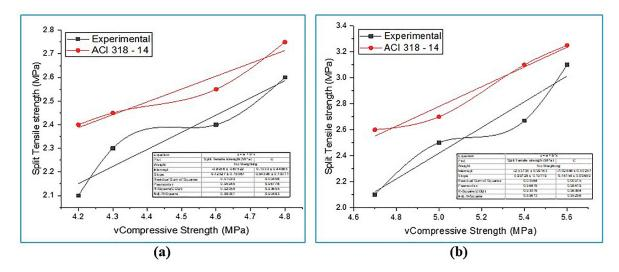
Figure 8: Comparison of the RSAC's split and compression tensile values after 28 days, (a) with and (b) with superplasticizer.
