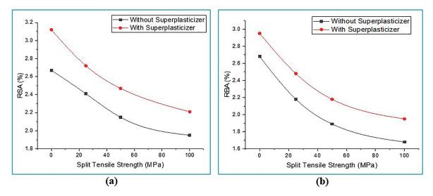
Figure 7: (a) RSAC and (b) RBAC - split tensile strength with/without superplasticizer after 28 days curing period.
