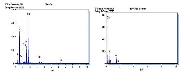
Figure 14: EDX images of (a) RBAC and (b) RSAC concrete mix with superplasticizer.
