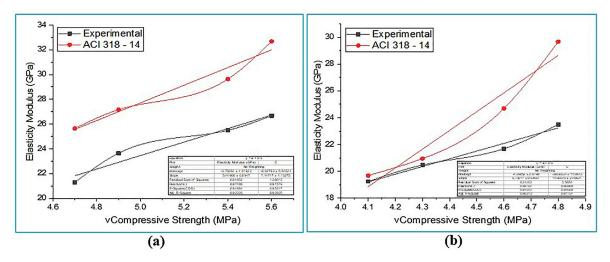
Figure 11: RSAC mixes - elasticity modulus and its relationship with/without superplasticizers.
