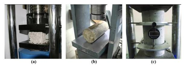
Figure 3: Laboratory setup of (a) compression, (b) split tensile and (c) elasticity modulus for concrete mixes.
