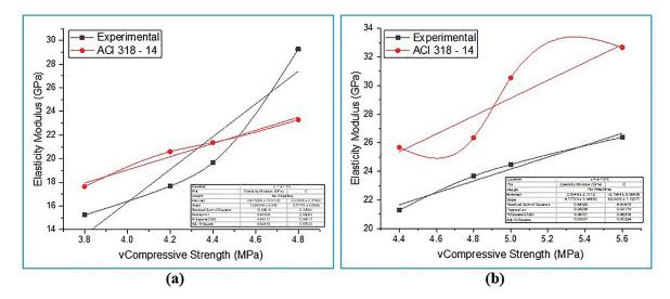
Figure 12: RBAC mixes - elasticity modulus and its relationship with/without superplasticizers.
