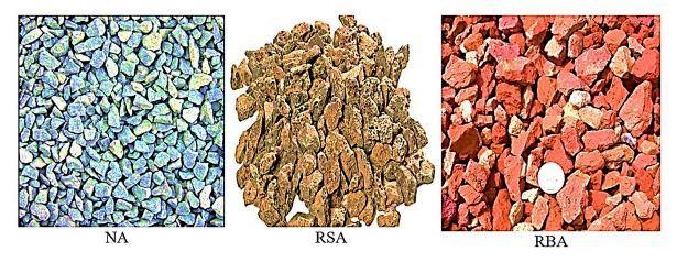
Figure 1: Types of coarse aggregates used for concrete mixes.
