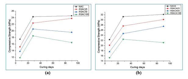
Figure 4: RSAC-compressive strength of cylinder specimens at different curing periods (a) without and (b) with superplasticizer.
