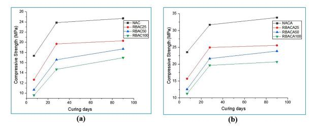
Figure 5: RBAC – compressive strength of cylinder specimens at different curing periods (a) without and (b) with superplasticizer.
