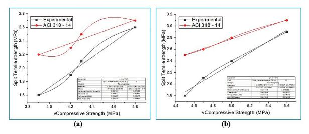
Figure 9: Comparison of the RBAC's split and compression tensile values after 28 days, (a) with and (b) with superplasticizer.
