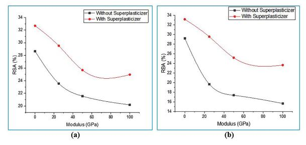
Figure 6: (a) RSAC and (b) RBAC – compressive strength with/without superplasticizer after 28 days of curing period.
