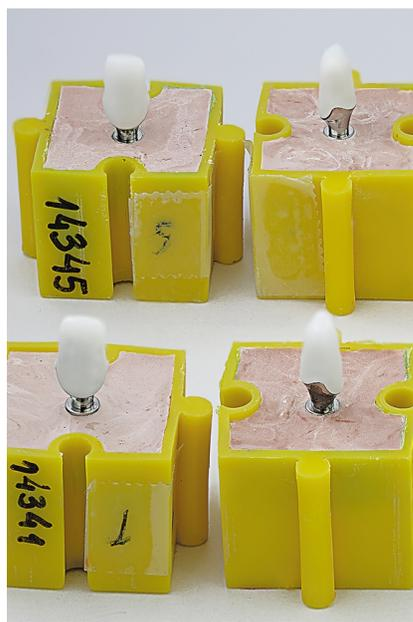
**Figure 2.** Zirconia copings on anatomic titanium abutment.
