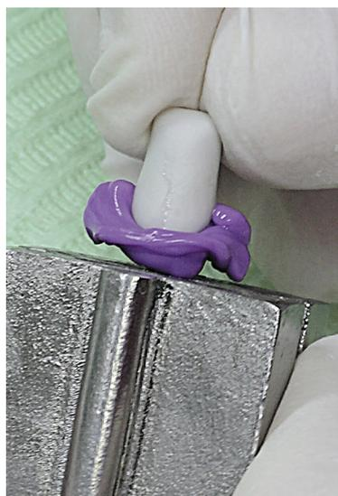
**Figure 4.** Zirconia coping cementation with silicone manually.
