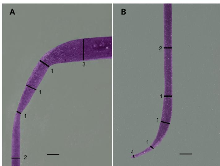
**Figure 6.** Standardization (original magnification ×100) used to measure the regions misfit. A: angular (1), linear (2), and incisal regions (3). B: angular (1), linear (2) and marginal regions (4). Perpendicular line drawn from abutment to internal surface of coping. Scale bar, 100 µm.
