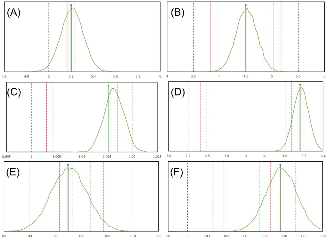
**FIGURE 1** - Measured values (green lines), specification limits (black lines), acceptance limits (red lines), and multivariate acceptance limits (blue lines) for ciprofloxacin ophthalmic solution (generic medicine). Legend: (A) volume (mL); (B) pH; (C) density (g/mL); (D) assay (mg/mL); (E) potency (%); and (F) drop test (mg/drop).
