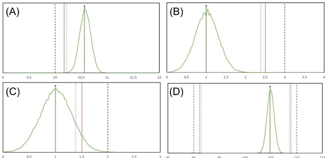
**FIGURE 3** - Measured values (green lines), specification limits (black lines), acceptance limits (red lines), and multivariate acceptance limits (blue lines) for acyclovir topical cream (generic medicine). Legend: (A) weight (g); bacteria count (CFU/g); (C) fungal count (CFU/g); and (D) assay (%).
