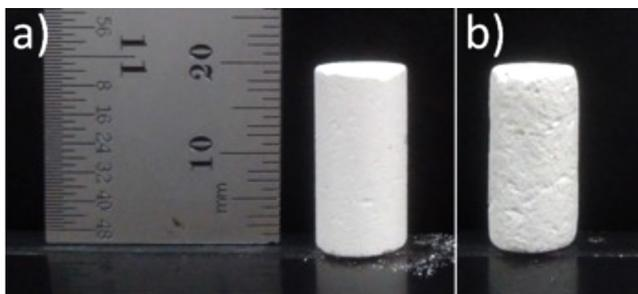
Figure 8: Images of samples: a) before conversion (gypsum/PHB); and b) after conversion (HAp/PHB).
