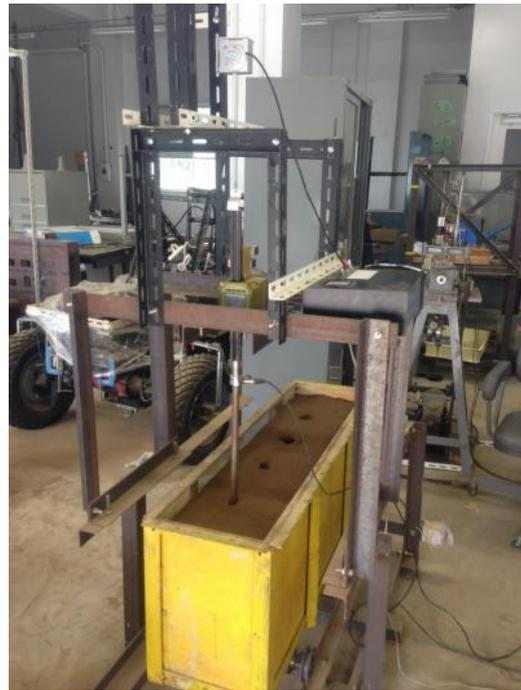
FIGURE 6. Locale photo of the penetration device.
