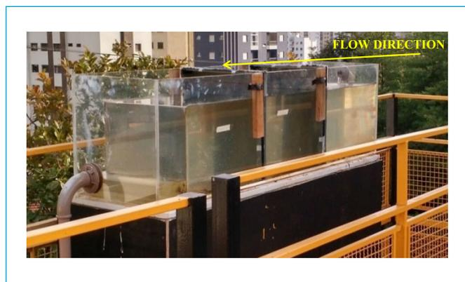
**Figure 2** - Acrylic channel used in the experiment with the turbidity barriers installed.
