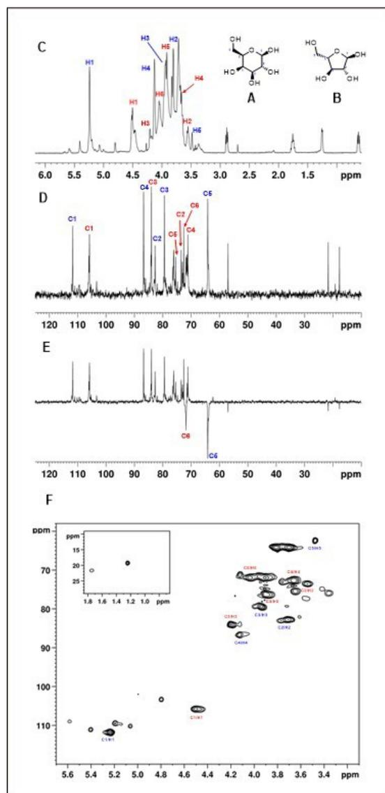
**Figure 3.** Unit structures (A) β-D-Galactopyranose and (B) α-L-Arabinofuranose; (C) <sup>1</sup>H NMR; (D) <sup>13</sup>C; (E) DEPT 135; and (F) HSQC. The chemical shifts in ppm of C and H refer to β-D-Galactopyranose shown in red, while to α-L-Arabinofuranose is shown in blue.
