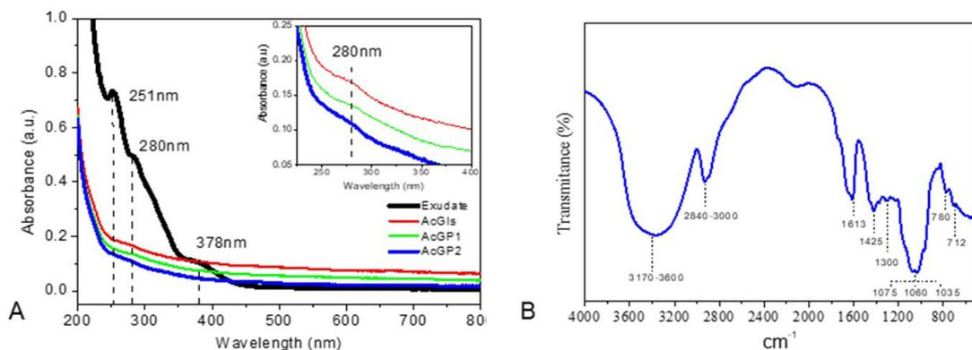
**Figure 1.** (A) Absorbance spectra in the Ultraviolet-Visible region of a 0.1% w/v aqueous solution of the exudate of *Amburana cearensis*, AcGIs, AcGP1, and AcGP2; (B) FTIR spectrum obtained for AcGP2 in KBr.
