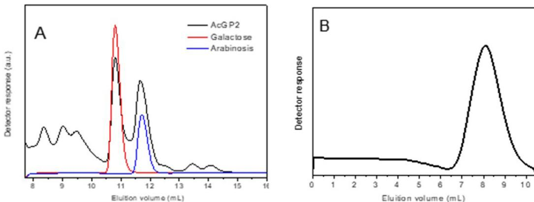
**Figure 2.** (A) HPLC graph to determine the main monomers of AcGP2; (B) GPC graph to determine the molar mass distribution of AcGP2.
