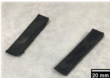
Figure 4 – Printed samples of LDPE-0.5%wtGO (left), LDPE-1.5%wtGO (right) - with extruder temperature of 240 °C and Print Bed of 20 °C - Layer Height: 0.2 mm - Filling density: 100% - Speed: 45 mm/s.
