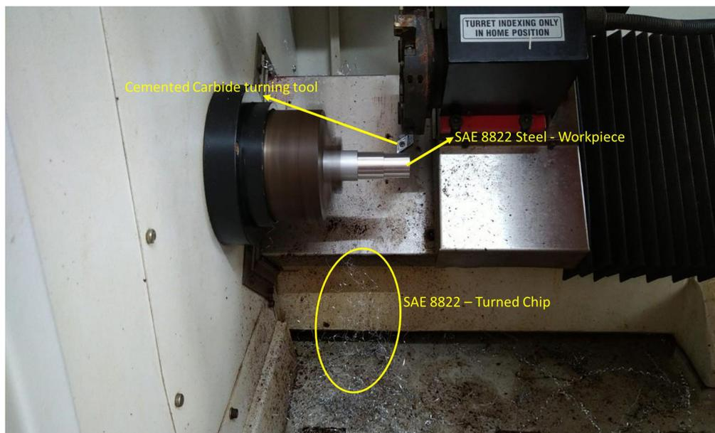
**Figure 1:** Experimental run - turning of SAE 8822 without coolant.
