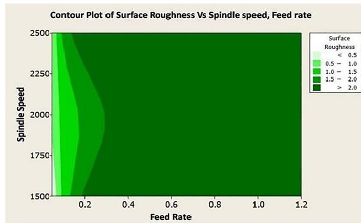
Figure 6: Contour plot for roughness ( $R_a$ ) versus spindle speed (A) and feed rate (B).
