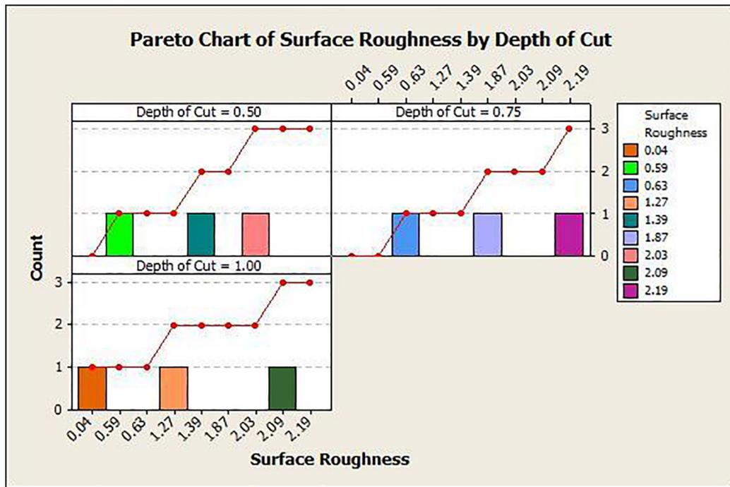
Figure 5: Pareto chart of surface roughness ( $R_a$ ) by depth of cut (C).
