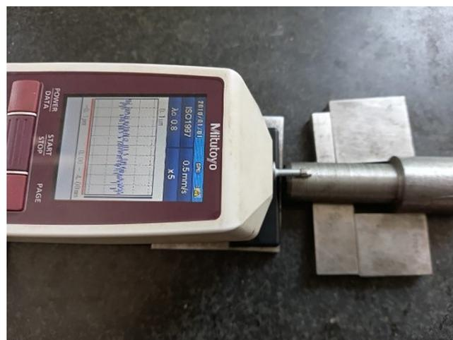
**Figure 2:** Surface roughness measurement of workpiece after turning.
