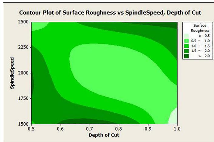
Figure 7: Contour plot for roughness ( $R_a$ ) versus spindle speed (A) and depth of cut (C).
