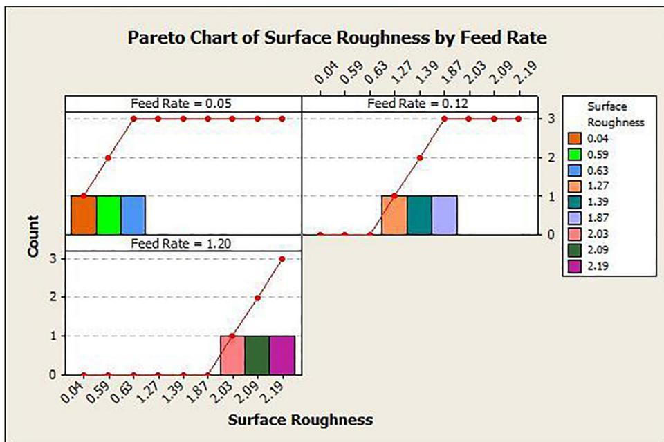
Figure 4: Pareto chart of surface roughness ( $R_a$ ) by feed rate (B).
