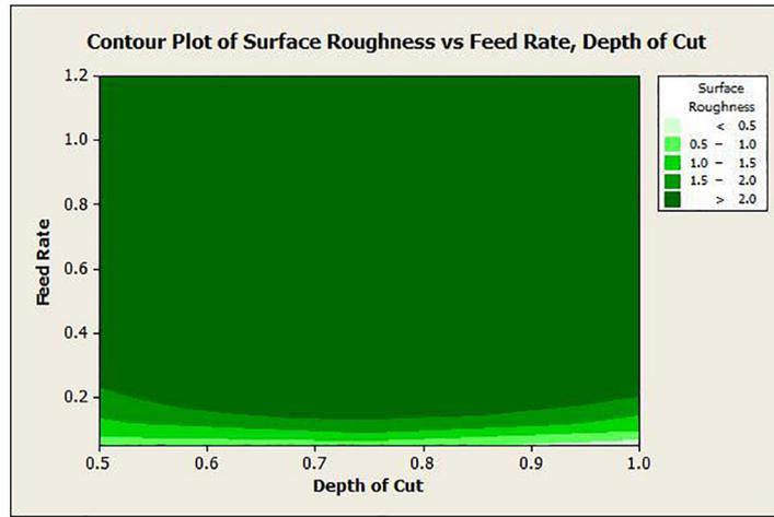
Figure 8: Contour plot for roughness ( $R_a$ ) versus feed rate (B) and depth of cut (C).
