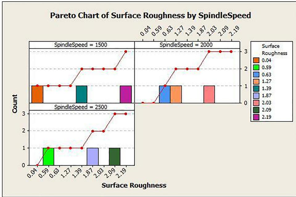
Figure 3: Pareto chart of surface roughness ( $R_a$ ) by spindle speed (A).
