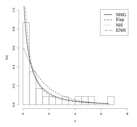
Figure 7 - Estimated for models fitted to the times between failures (thousands of hours) of secondary reactor pumps.
