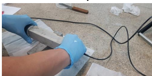
Figure 10 - Test using the dynamic modulus of elasticity method
