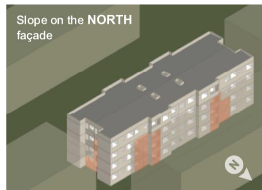
Figure 16 - ROCs not meeting the requirements of the proposed Section 13 of NBR 15575-1 (ABNT, 2024a) under four solar orientations in Recife
