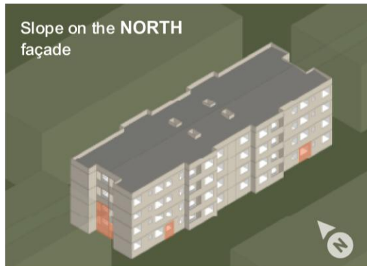
Figure 16 - ROCs not meeting the requirements of the proposed Section 13 of NBR 15575-1 (ABNT, 2024a) under four solar orientations in Recife
