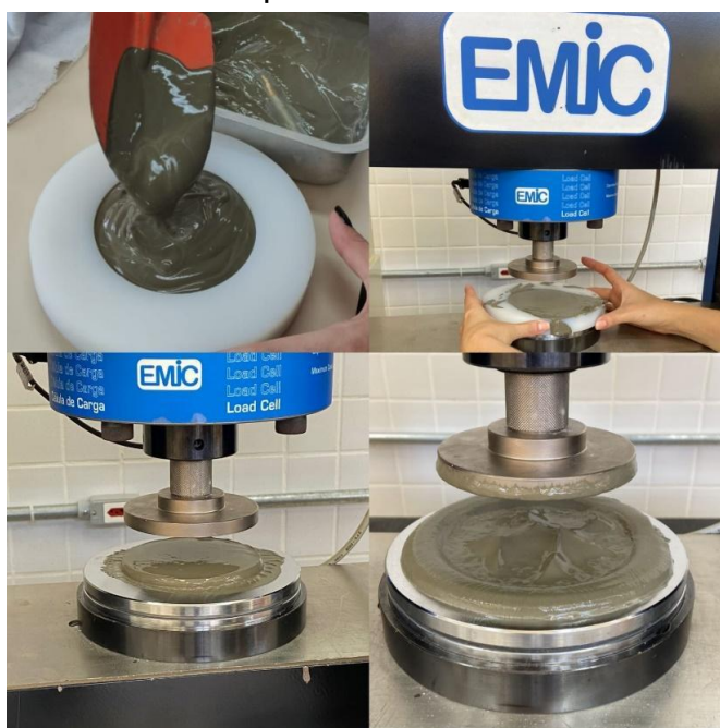
Figure 4 - Squeeze-flow test of the cement paste
