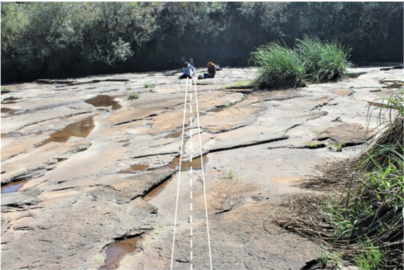
Figure 2 Cross section analyzed in the study (dashed line), with a 50 cm width strip where the strength measurements were obtained.
