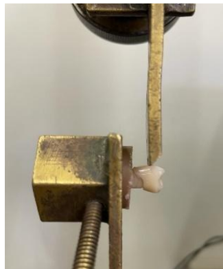
Figure 3. Position of the tooth/resin set for the shear bond test.
