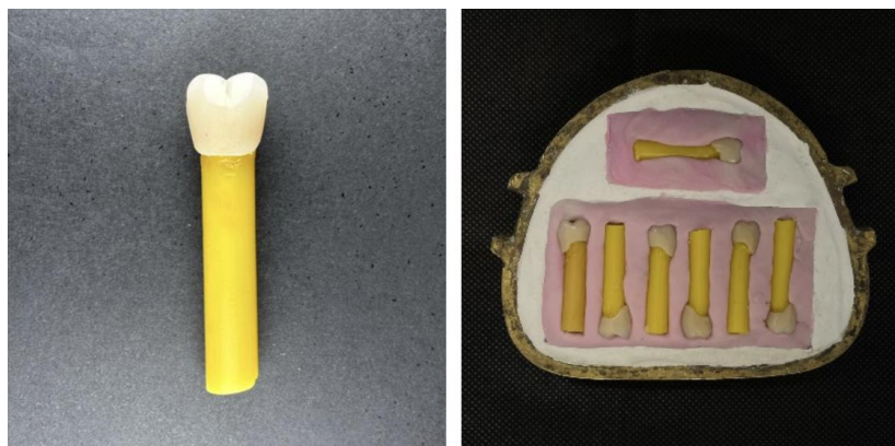
Figure 1. Tooth/wax stick set and inclusion in the metal flask.
