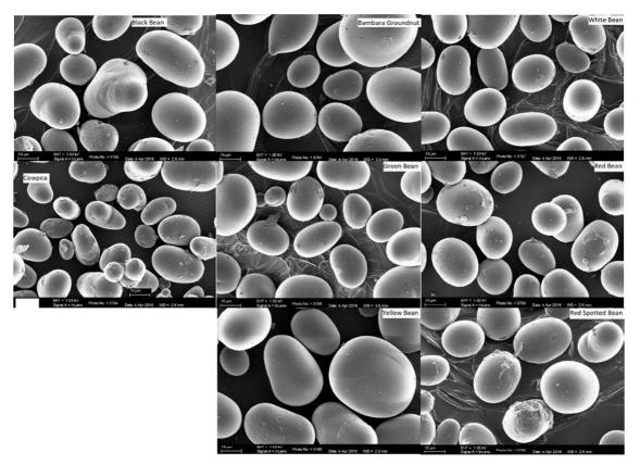
Figure 2. Scanning electron micrographs of eight Cameroonians native legume starches.
