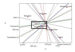
Figure 5. Principal component analysis represented on two principal components.
