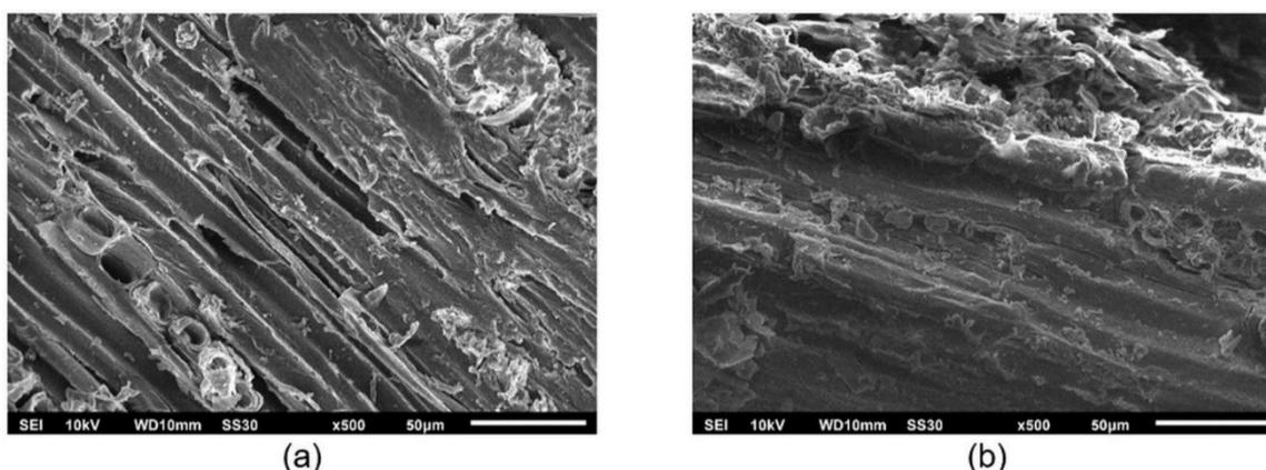
**Figure 3.** Morphologies of sappan wood surface after extraction for (a). UAE method (U60), (b). Soxhlet method (S60).
