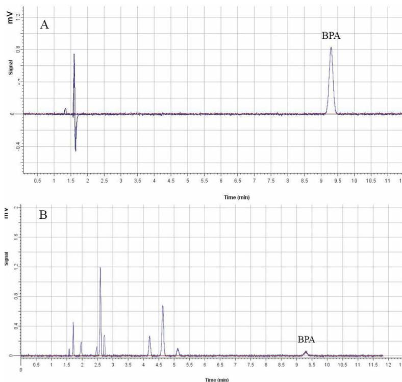
**FIGURE 2** – Typical chromatograms obtained from a standard solution of BPA (0.5 µg/mL) (A) and a sample of makkous (B).
