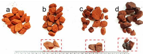
Figure 3: Image of the aggregates before sintering (a) and after the sintering of samples S5 (b), S15 (c), and S25 (d).
