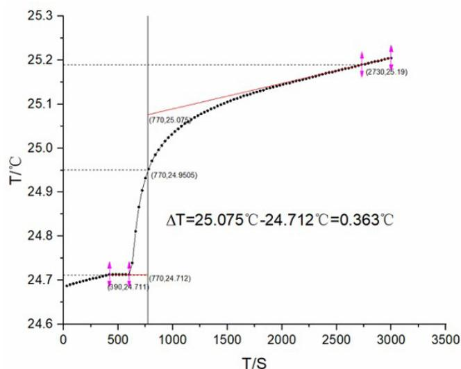
Figure 1.  $\Delta T$  curve of Reynolds temperature of cinnamon.
