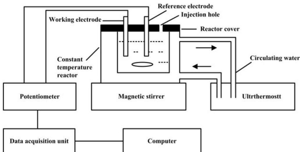
Figure 1. Schematic diagram of nonlinear chemical oscillation system.
