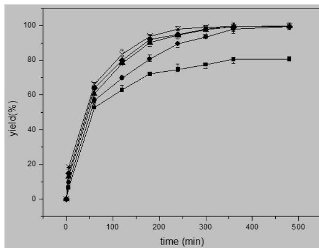
**Figure 3.** Effect of molar ratio of vinyl acetate to citronellol. Reaction conditions: citronellol, 100 mmol/L; lipase, 10 mg/mL; temperature, 40 °C; speed of agitation, 200 r/min; (■) 1:1, (●) 2:1, (▲) 3:1, (◆) 4:1, (×) 5:1.
