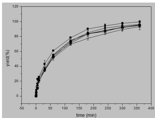
**Figure 9.** Effect of concentration of product. Reaction conditions: citronellol, 100 mmol/L; molar ratio of vinyl acetate to citronellol, 3:1; lipase, 10 mg/mL; temperature, 40 °C; speed of agitation, 200 rpm; (■) 0 mmol/L, (●) 50 mmol/L, (▲) 100 mmol/L, (◆) 150 mmol/L, (★) 200 mmol/L, (×) 250 mmol/L.
