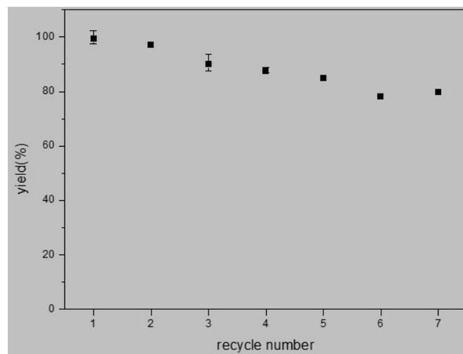
**Figure 11.** Reuseability of lipase. Reaction conditions: citronellol, 100 mmol/L; molar ratio of vinyl acetate to citronellol, 3:1; lipase, 10 mg/mL; temperature, 40 °C; speed of agitation, 200 r/min; reaction time, 6 h.
