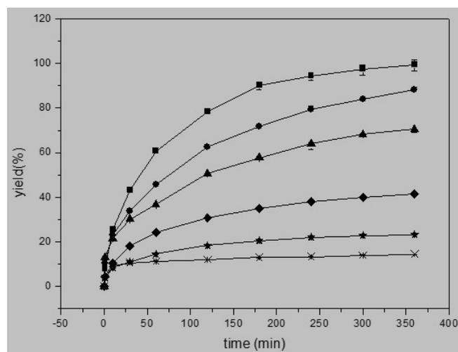
**Figure 10.** Effect of additional water. Reaction conditions: citronellol, 100 mmol/L; molar ratio of vinyl acetate to citronellol, 3:1; lipase, 10 mg/mL; temperature, 40 °C; speed of agitation, 200 rpm; (■) 0% (v/v), (●) 0.2% (v/v), (▲) 0.5% (v/v), (◆) 1% (v/v), (★) 2% (v/v), (×) 5% (v/v).
