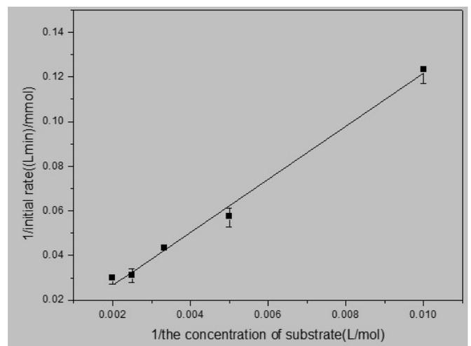
**Figure 8.** Lineweaver-Burk plot. Reaction conditions: molar ratio of vinyl acetate to citronellol, 3:1; lipase, 10 mg/mL; temperature, 40 °C; speed of agitation, 200 r/min.
