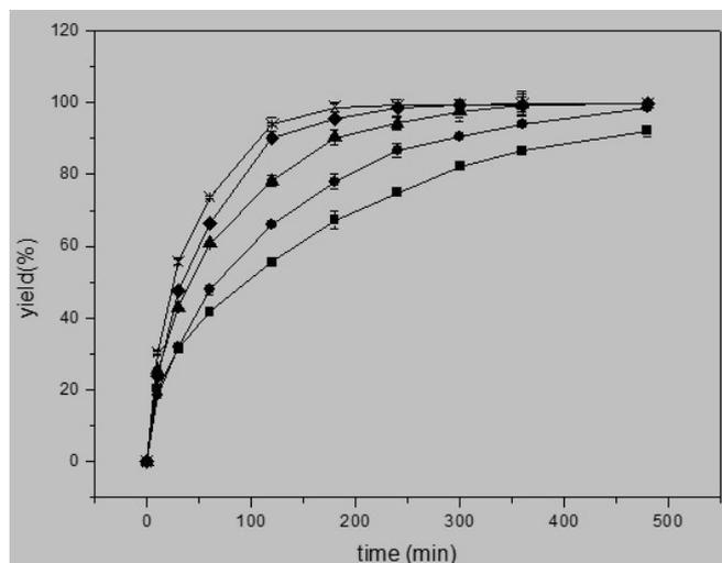
**Figure 4.** Effect of temperature. Reaction conditions: citronellol, 100 mmol/L; molar ratio of vinyl acetate to citronellol, 3:1; lipase, 10 mg/mL; speed of agitation, 200 r/min; (■) 20 °C, (●) 30 °C, (▲) 40 °C, (◆) 50 °C, (×) 60 °C.
