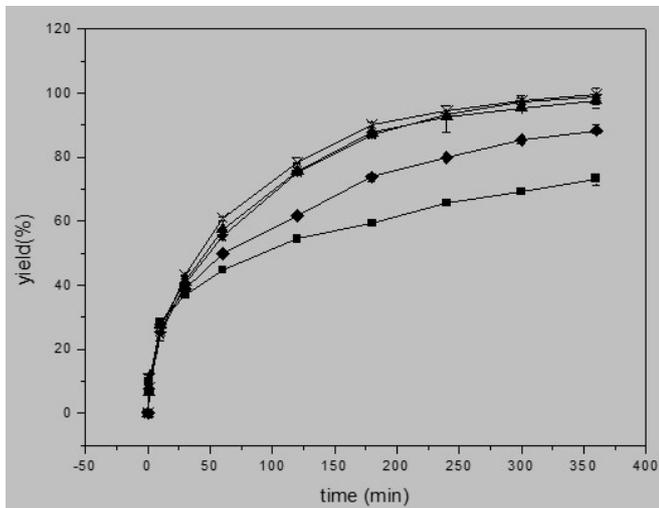
**Figure 6.** Effect of speed of agitation. Reaction conditions: citronellol, 100 mmol/L; molar ratio of vinyl acetate to citronellol, 3:1; lipase, 10 mg/mL; temperature, 40 °C; (■) 50 r/min, (◆) 100 r/min, (▲) 150 r/min, (×) 200 r/min, (★) 250 r/min.
