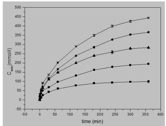
**Figure 7.** Effect of concentration of substrate. Reaction conditions: molar ratio of vinyl acetate to citronellol, 3:1; lipase, 10 mg/mL; temperature, 40 °C; speed of agitation, 200 rpm; (■) 100 mmol/L, (●) 200 mmol/L, (▲) 300 mmol/L, (★) 400 mmol/L, (×) 500 mmol/L.
