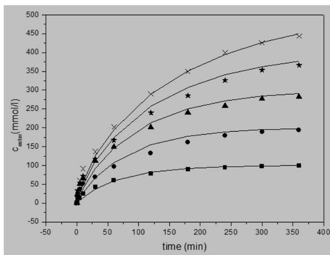
**Figure 13.** Comparison of simulated values with the experimental data. For the initial concentration of citronellol, the experimental values are represented as points: (■) 100 mmol/L, (●) 200 mmol/L, (▲) 300 mmol/L, (★) 400 mmol/L, (×) 500 mmol/L. The simulated values are represented by the trend lines.
