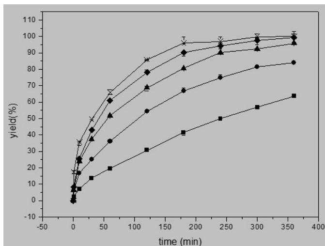
**Figure 5.** Effect of enzyme loading. Reaction conditions: citronellol, 100 mmol/L; molar ratio of vinyl acetate to citronellol, 3:1; temperature, 40 °C; speed of agitation, 200 r/min; (■) 2.5 mg/mL, (●) 5 mg/mL, (▲) 7.5 mg/mL, (◆) 10 mg/mL, (×) 12.5 mg/mL.
