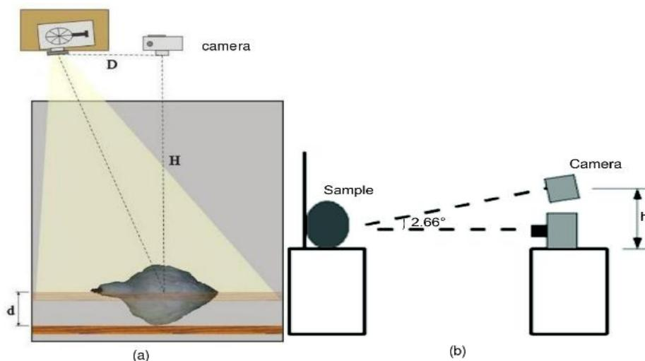
FIGURE 1. Experimental setup used for image acquisition, showing black painted vertical board moved by half of animal width, in (a) a top view, and in (b) a lateral view.
