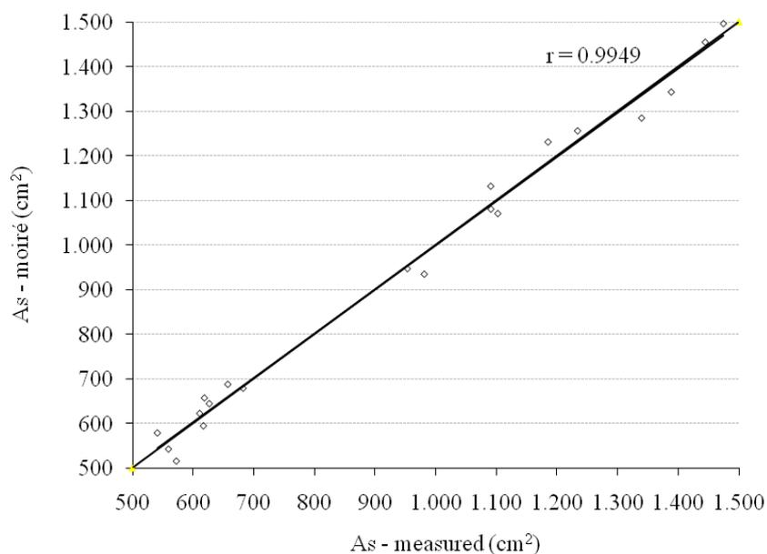
FIGURE 5. Comparison between surface area (SA) determined by the conventional method and SA determined by the *moiré* technique with application of correction factor.
