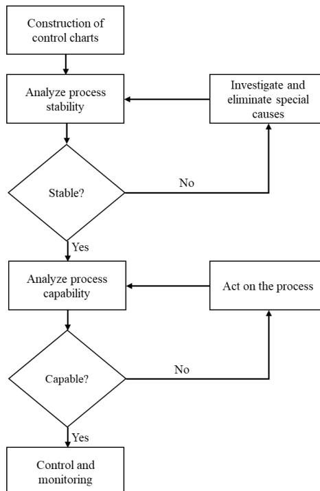
**Figure 1.** Schematic of Statistical Process Control. Source: Álvarez et al. (2015).
