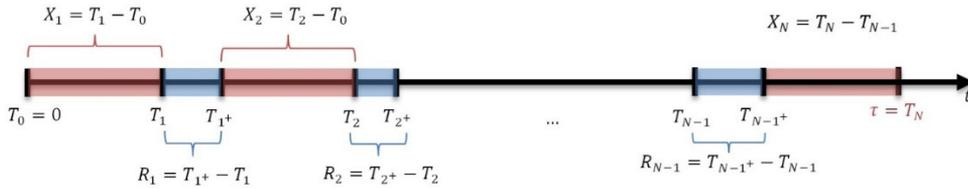
**Figure 3.** Illustrative graphic to represent the times in the operation and maintenance of a system.
