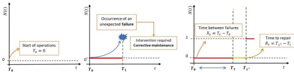
**Figure 4.** Dynamics illustrating the occurrence of failure and maintenance intervention in a repairable system (Medeiros et al., 2022).
