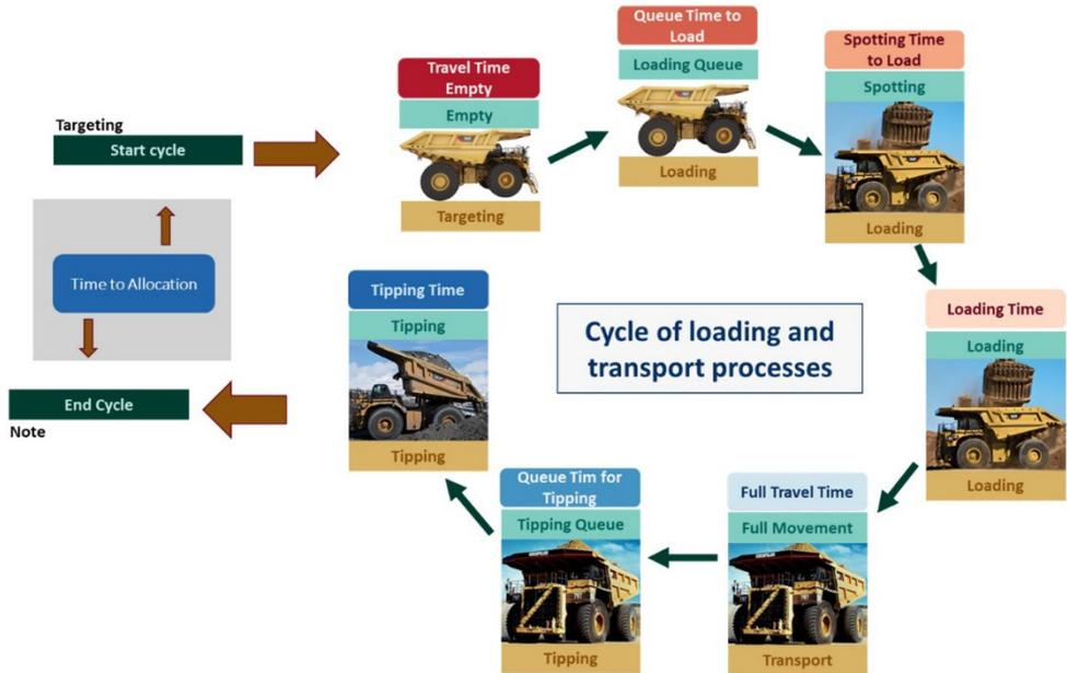
Figure 1. Cycle of loading and transportation processes.
