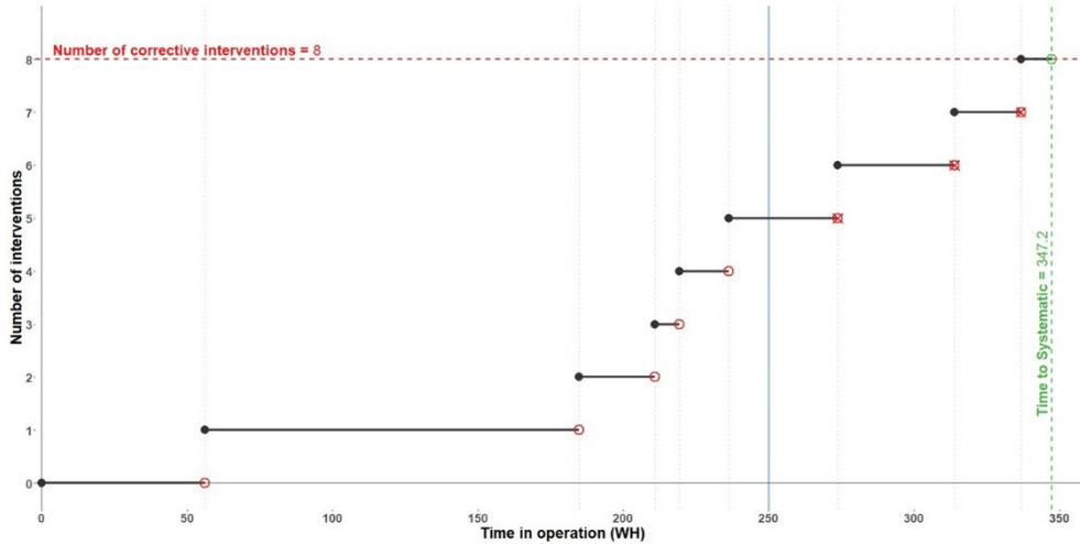
Figure 10. Counting processes applied to TAG 5513 truck for first systematic intervention.
