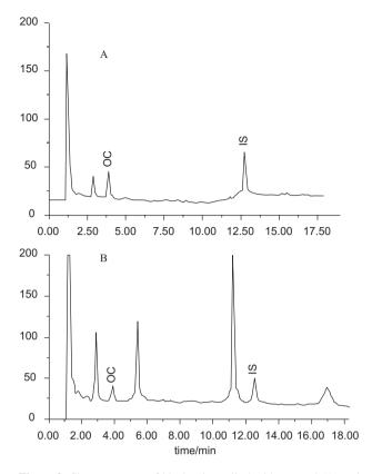
**Figure 3.** Chromatograms of blank urine spiked with *o*-cresol (A) and from a sample obtained from a worker exposed to solvents in an automotive repair and repainting shop (B), both added with internal standard, *p*-nitroaniline, and extracted by CW/DVB fiber.
