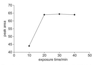
Figure 1. Peak areas *versus* extraction time obtained with CW/DVB fiber for o-cresol in urine spiked with 2 mg L<sup>-1</sup> and stirred.
