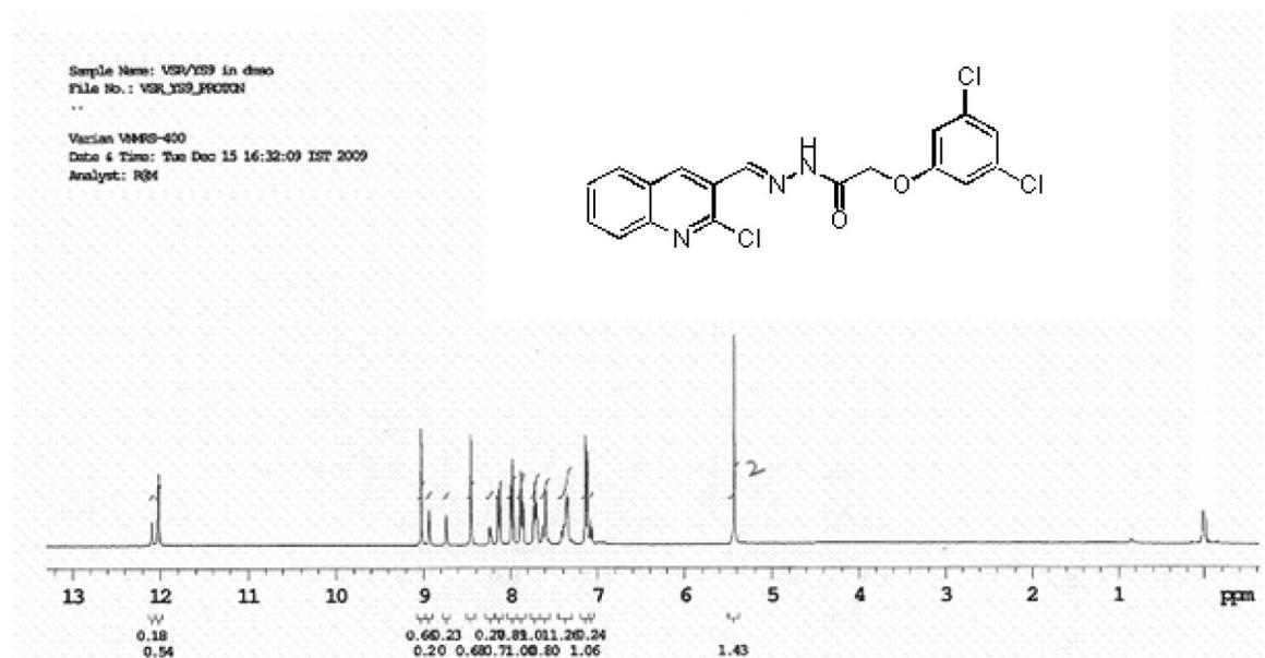
Figure S5.  $^1\text{H}$  NMR of compound **3e** in  $\text{DMSO-}d_6$ .
