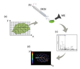
**Figure 1.** Sequential steps in a DESI-MSI procedure: (a) tracing lines on the entire sample surface in the y direction (each line is composed by a number of spots or pixels); (b) scanning the entire surface (line after line) with the fine spray (stream of charged microdroplets); (c) acquiring and storing the mass spectra (one for each pixel); (d) conversion of the mass spectra data into 2D images.
