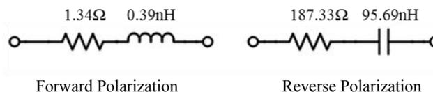
Fig. 2. The equivalent circuit model for forward and reverse biased PIN diode.
