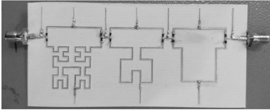
Fig. 5. Fabricated fractal-based phase shifter.
