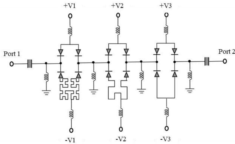
Fig. 3. Fractal phase shifter using PIN diodes.
