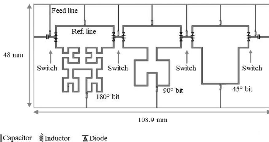
Fig. 4. Proposed fractal-based phase shifter.
