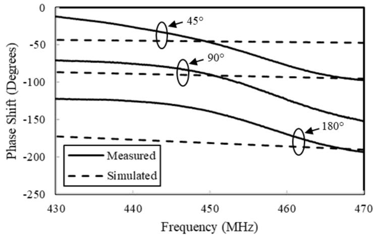
Fig. 6. Simulated and measured phase shift versus frequency.
