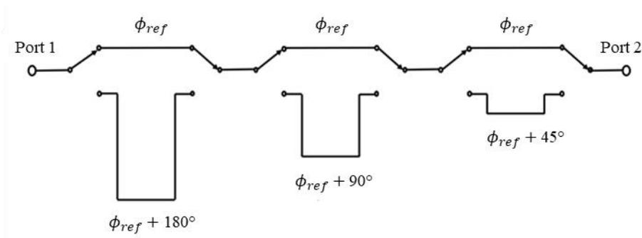
Fig. 1. 3-bit switched line phase shifter.
