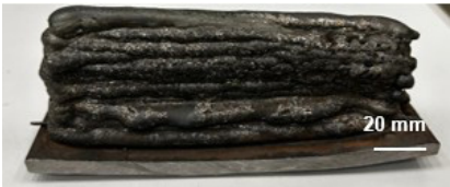
Figure 3. Metallic wall obtained by AM through the GTAW-WAAM process, evidencing the layer-by-layer formation and the final geometry of the deposited structure.
