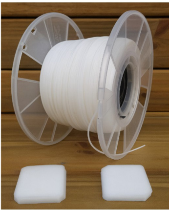
Figure 1. (a) Schematic of polypropylene composite fabrication with antimicrobial additives; (b) Extruded filament spool (~500 g, 1.75 mm diameter) of polypropylene containing 10% ZnO-based glassy ceramic additive (Si–Na–Al matrix), and corresponding 3D-printed test specimens (2 × 50 × 50 mm).
