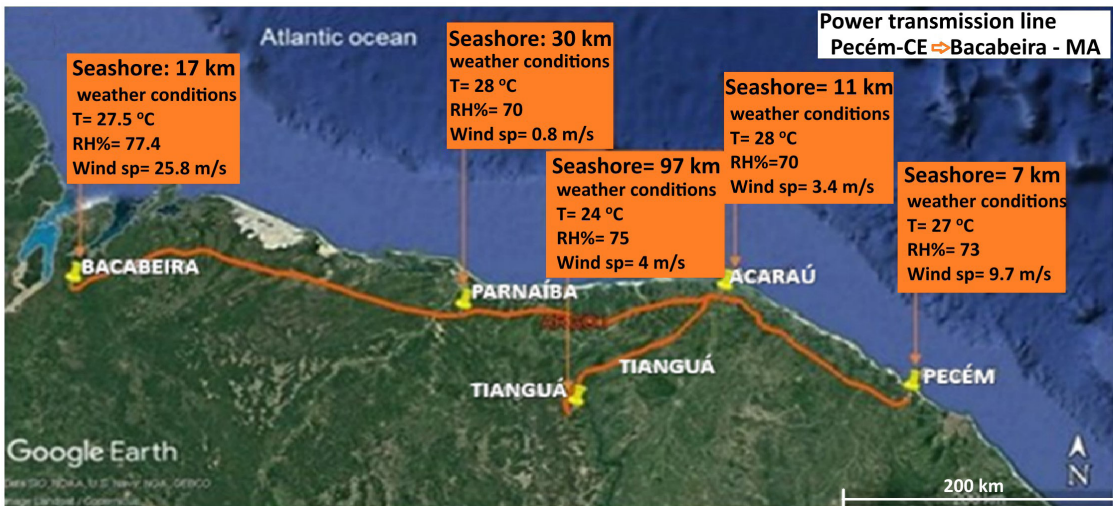
Figure 1. Map of the 1,150 km transmission line (TL) studied for atmospheric corrosivity assessment, spanning from Pecém II substation (CE) to Bacabeira substation (MA), through Acaraú (CE), Tianguá (CE), and Parnaíba (PI). The figure shows distances from the coastline (7–97 km) and local meteorological conditions at each exposure site.
