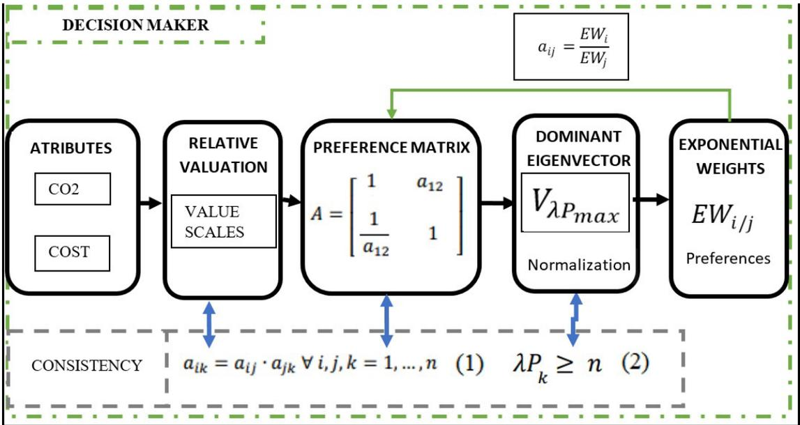
Figure 2. Analytic Hierarchy Process (AHP) applied to the Argentine productive chain. Source: The author.
