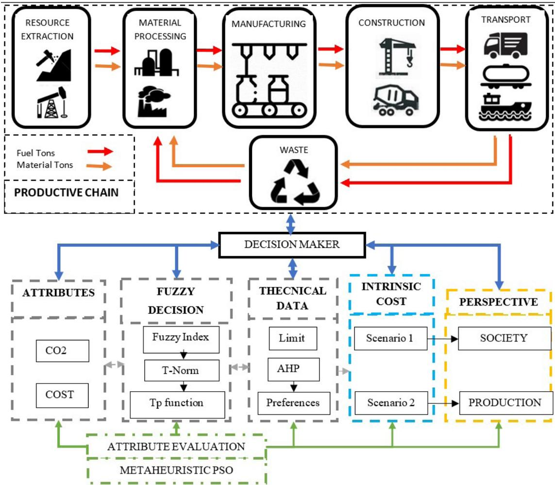
Figure 1. Life Cycle Analysis (LCA) model applied to the Argentine Productive Chain (APC), Analytic Hierarchy Process (AHP) and marginal evaluation model by means of intrinsic cost. Source: The author.
