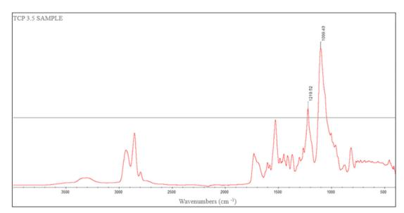
Figure 7. FTIR graphic from TCP3.5 reaction cured with 4,4'-methylenebis(2-chloroaniline)
