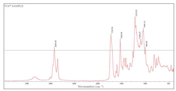
Figure 6. FTIR graphic from TC6\* reaction cured with castor oil
