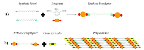
Figure 1. a) Reaction between isocyanate and polyol forming urethane prepolymer b) Reaction between urethane prepolymer and chain extender forming urethane prepolymer
