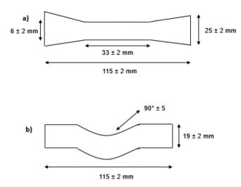
Figure 3. Measurements of specimens to tensile stress, elongation and tear strength
