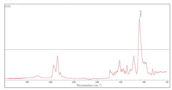
Figure 8. FTIR graphic from STD reaction cured with 4,4'-methylenebis(2-chloroaniline)
