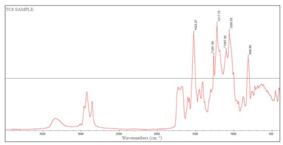
Figure 5. FTIR graphic from TC6 reaction cured with 4,4'-methylenebis(2-chloroaniline)
