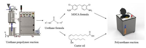
Figure 2. Sketch of reactions considering urethane prepolymer with MOCA (4,4'-methylenebis(2-chloroaniline) and castor oil
