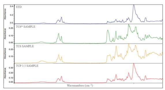
Figure 4. ATR spectra for STD, TC6\*, TC6 and TCP3.5 samples
