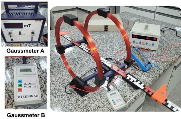
**Figure 4:** Used gaussmeters (left) and complete setup. The mobile phone and probes are placed on the middle point of the Helmholtz coil.
