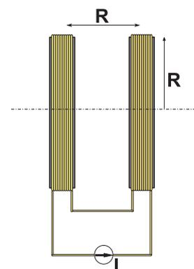
Figure 3: Schematic of a Helmholtz coil, excited by a current source with amplitude  $I$ .
