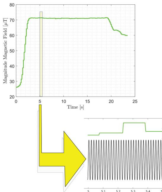
**Figure 10:** AC response of the coil. Inset shows a zoomed-in sector, alongside the expected oscillatory curve, not captured by the sensor.
