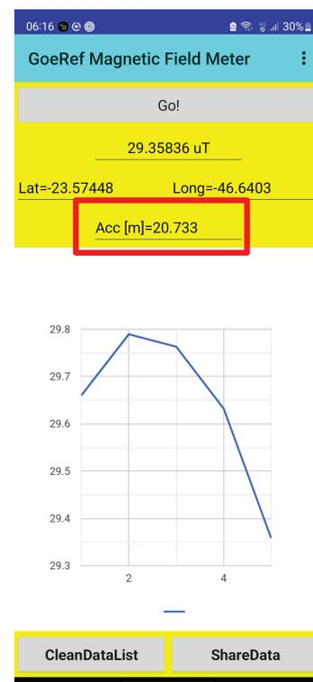
**Figure 5:** Screenshot of the magnetic field meter. The accuracy is shown in the red box.
