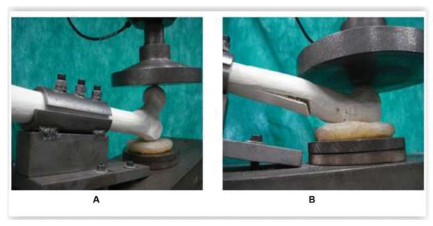
Fig. 3 Synthetic model in group B - (A) synthetic femur model fixed on the device during the test, demonstrating the position, and (B) after the test, presenting a longitudinal fracture.
