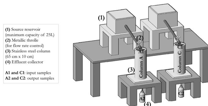
Figure 5. General scheme of soil column tests for this experiment.
