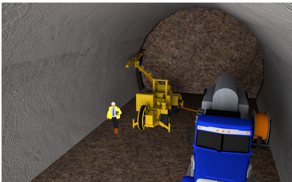
Figure 5 - The cycle proposes the introduction of a perimeter cutting stage executed by HPAWJ technology.
