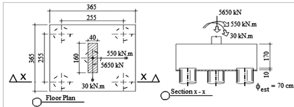
Figure 9 - Example 2 - Pile cap original design with loads values.
