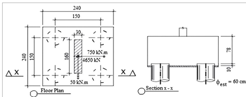
Figure 7 - Example 1 - Best design for CO<sub>2</sub> emission.
