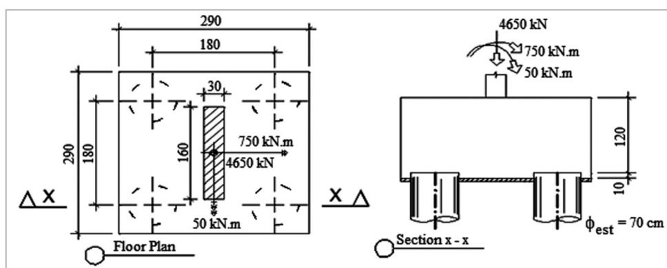
Figure 4 - Example 1 - Pile cap original design with loads values.
