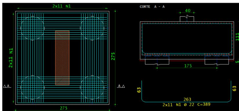
Figure 13 - Example 2 - Validation of the optimized pile cap design (adapted from TQS v.22 (2022)).
