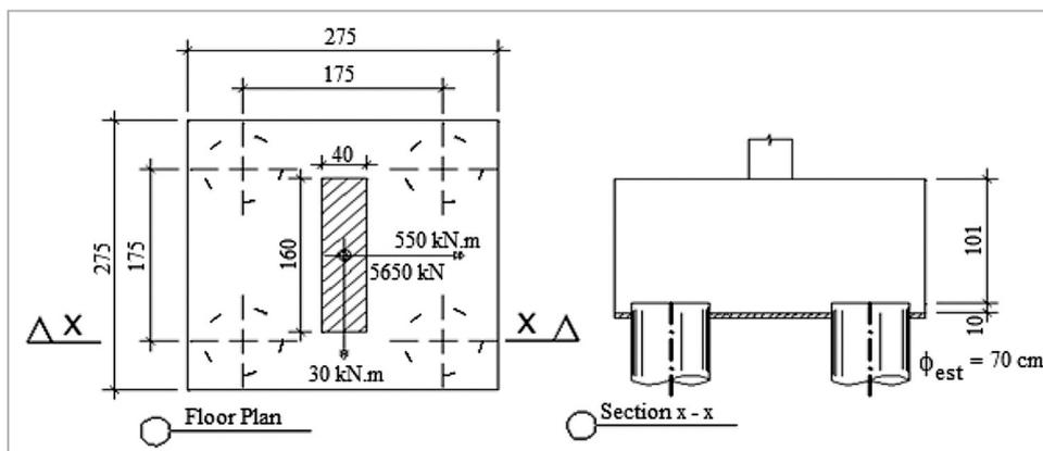
Figure 12 - Example 2 - Best design for CO<sub>2</sub> emission.
