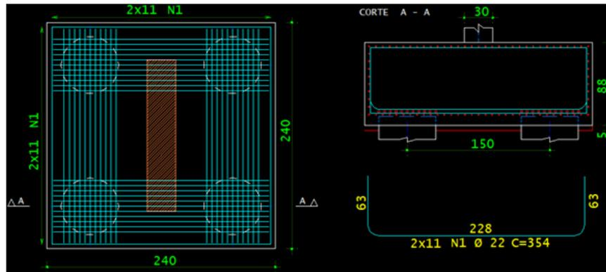
Figure 8 - Example 1 - Validation of the optimized pile cap design (adapted from TQS v.22 (2022)).
