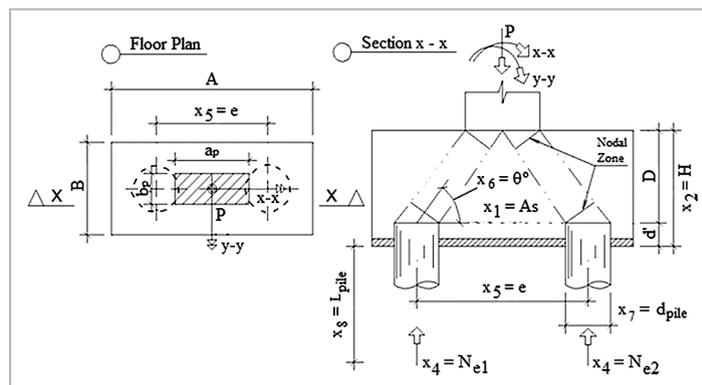
Figure 1 - Problem variables of the strut-and-tie method for a two-pile cap.
