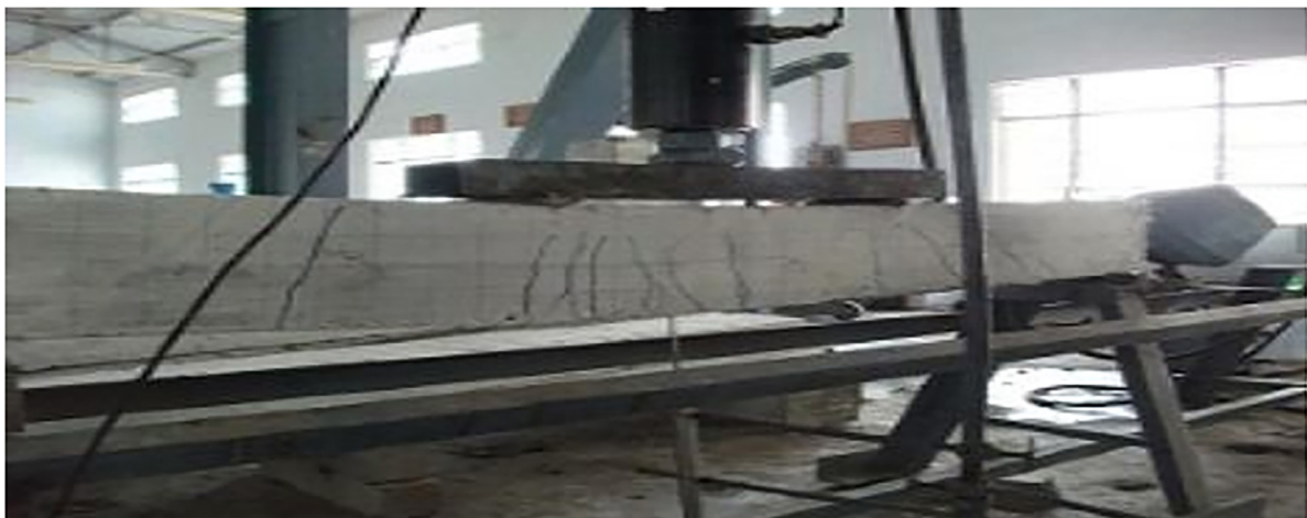
Figure 4: Cyclic loading of beams.
