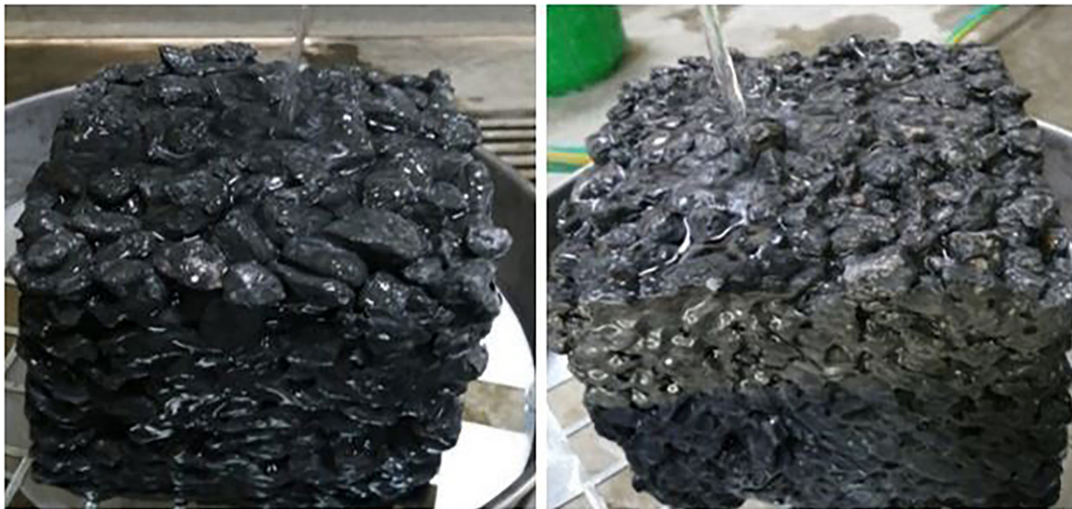
Figure 11: Image of the concrete while testing for permeability.
