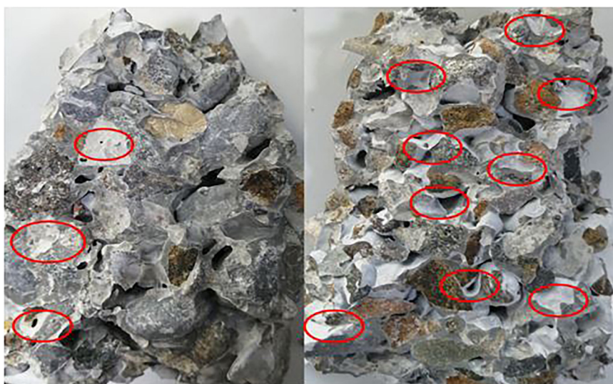
Figure 15: Voids in pervious concrete with 20 mm coarse aggregate and 0.4 water ratio on left and 0.3 water ratio on right.
