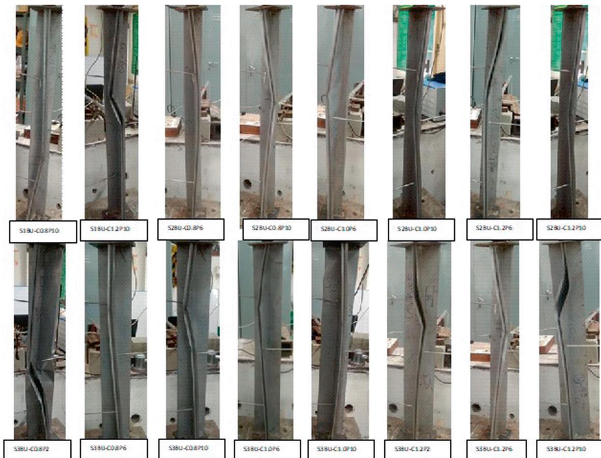
Figure 10: Deformed shapes of specimen after experiments.
