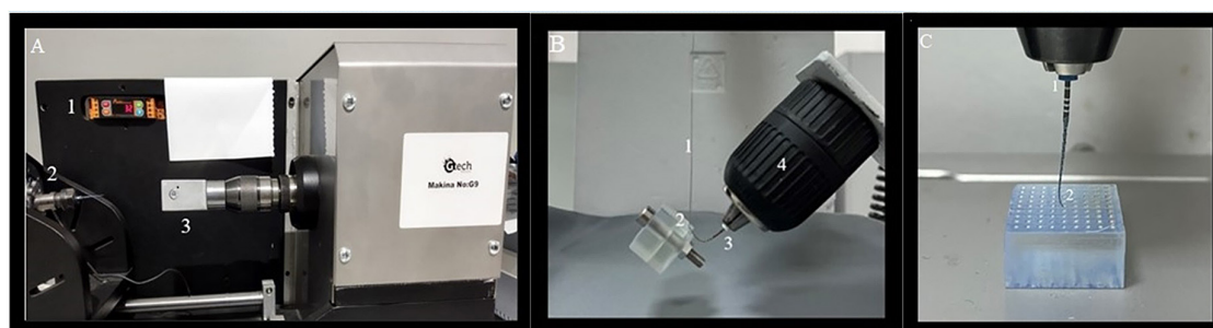
Figure 1: A: Torsional resistance test assembly. The instrument is affixed to a Jacobs mandrel by the cable and clamped 3 mm from their tips using a Chuck (1: Torque display screen, 2: Fixation area of shaft 3: Fixation area of the 3 mm tip of the file.), B: Bending test setup: (1: Wire used to pull the instrument, 2: Clamps to fix the instrument tip, 3: Jacobs chunk), C: Buckling test setup (1: Jacobs chunk, 2: base assembled to perform the buckling test).
