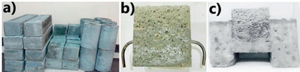
**Figure 6:** Test samples: (a) cubes, cylinders, and prisms, (b) specimen with nails, and (c) bond strength specimen.
