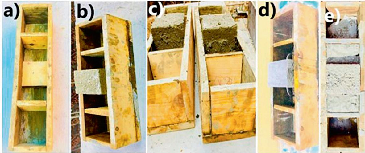
**Figure 3:** Molding and casting for bond strength test specimens (a) wooden molds, (b) casting specimens with old concrete, (c) casting specimens with agent material, (d) casting specimens with nails, and (e) casting specimens with new concrete.
