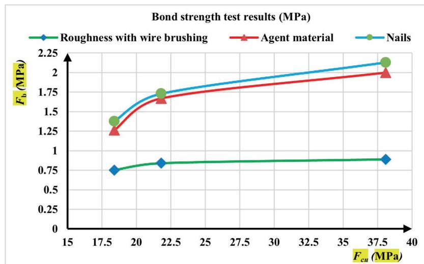
**Figure 7:** Average bond strength test results for different treatment cases.
