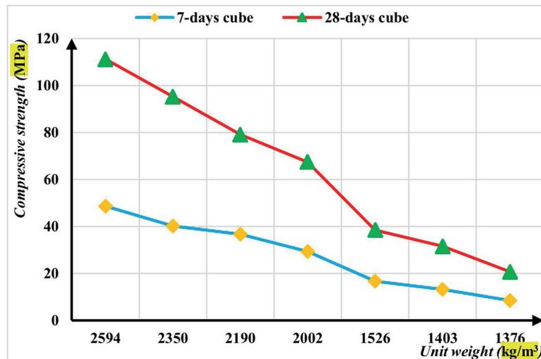
Figure 11: Relationship between unit weight and cube compressive strength.
