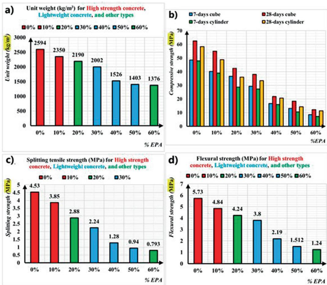
Figure 10: Effect of changing perlite replacement ratio on (a) unit weight, (b) compressive strength, (c) indirect-tensile strength, and (d) flexural strength.
