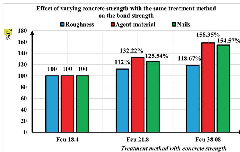
Figure 13: Effect of changing concrete strength with the same treatment method on the bond strength
