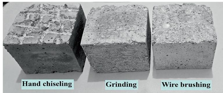
**Figure 4:** Surface preparation for specimens with different roughness techniques.
