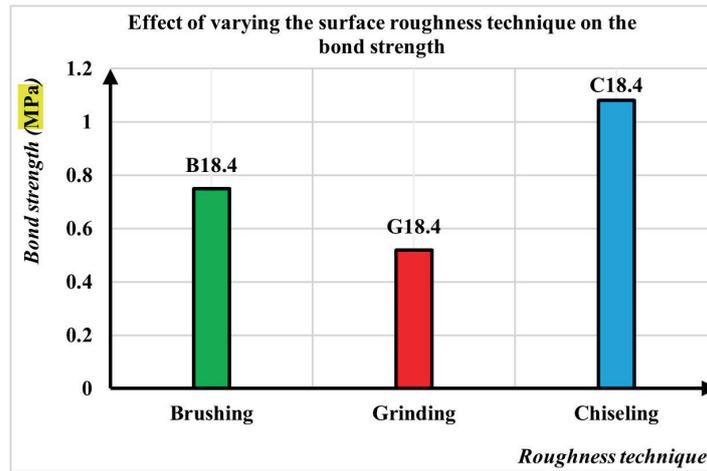
Figure 12: Effect of changing the surface roughness technique on the bond strength.
