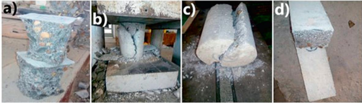
Figure 8: Failure mode for; (a) cubes for compression test, (b) cylinders for compression test, (c) cylinders for splitting tensile test, and (d) prisms for flexural test.
