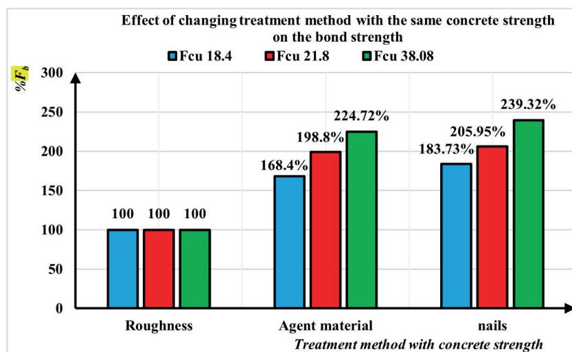
**Figure 14:** Effect of changing treatment method with the same concrete compressive strength on the bond strength.
