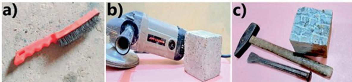
**Figure 5:** Tools used for surface preparation process: (a) hand wire brushing, (b) grinding, and (c) hand chiseling.
