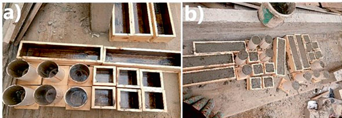
Figure 2: Molding and casting for cube, cylinder, and prismatic specimens (a) wooden molds, and (b) casting specimens.
