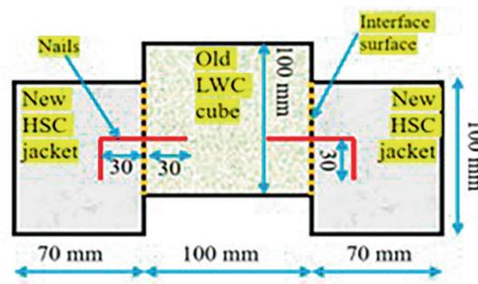
Figure 1: Dimensions for bond strength test specimens.
