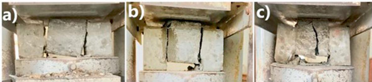
Figure 9: Failure for bond strength test specimens in case of; (a) roughness, (b) agent material, and (c) nails.
