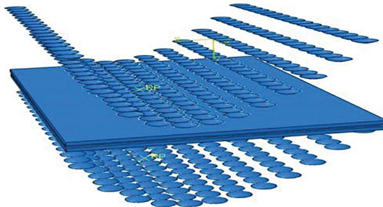
**Figure 6:** Multi-point forming finite element model.
