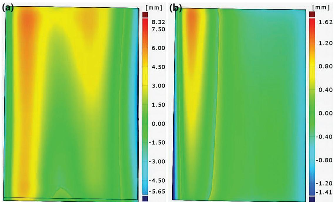
Figure 10: Error distribution cloud of test parts.
