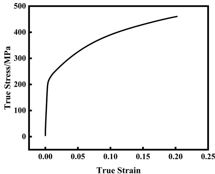
**Figure 4:** Stress-strain curve of corrosion-resistant aluminum alloys used in this paper.
