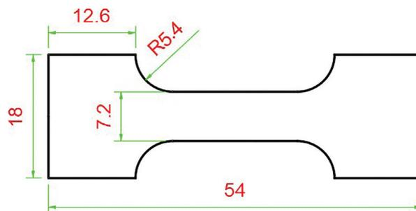
Figure 2: Dimensional parameters of specimens.
