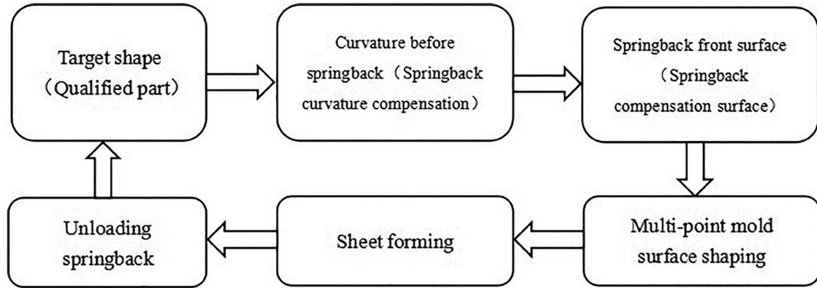
Figure 5: Springback compensation method.
