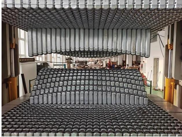
Figure 8: Multi-point forming press.
