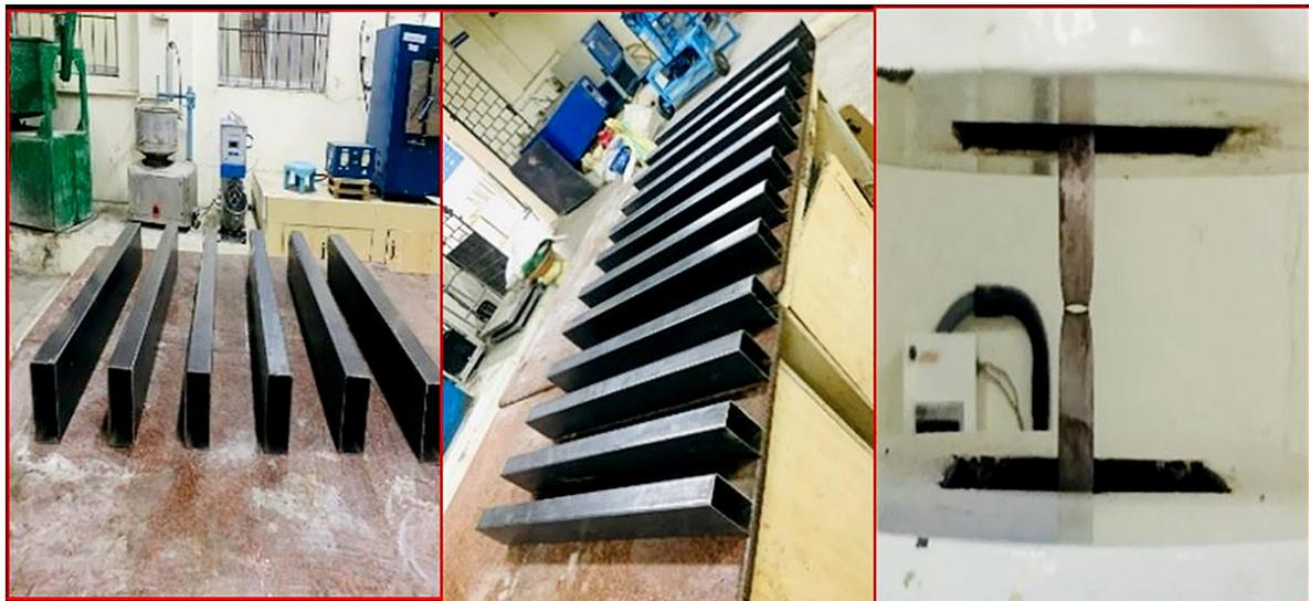
**Figure 2:** Light gauge steel tube and tensile coupon test.
